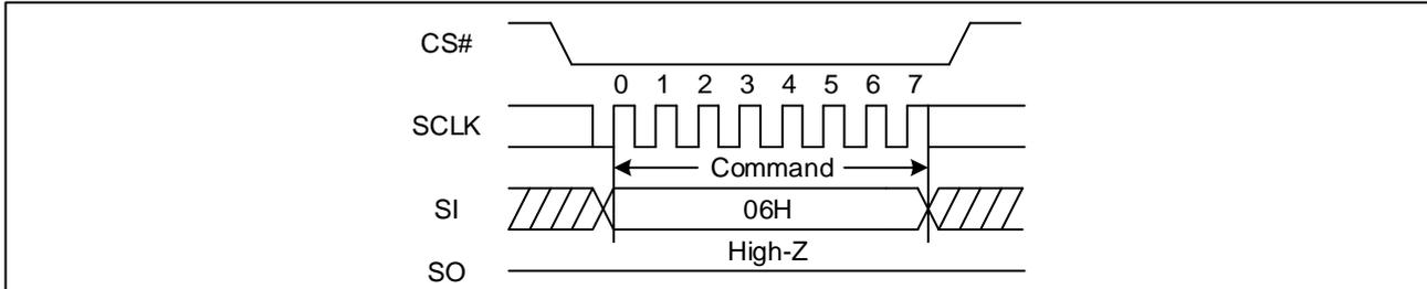
**Figure 4. Write Enable Sequence Diagram (QPI)**
