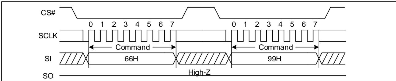
**Figure 49. Enable Reset and Reset command Sequence Diagram (QPI)**
