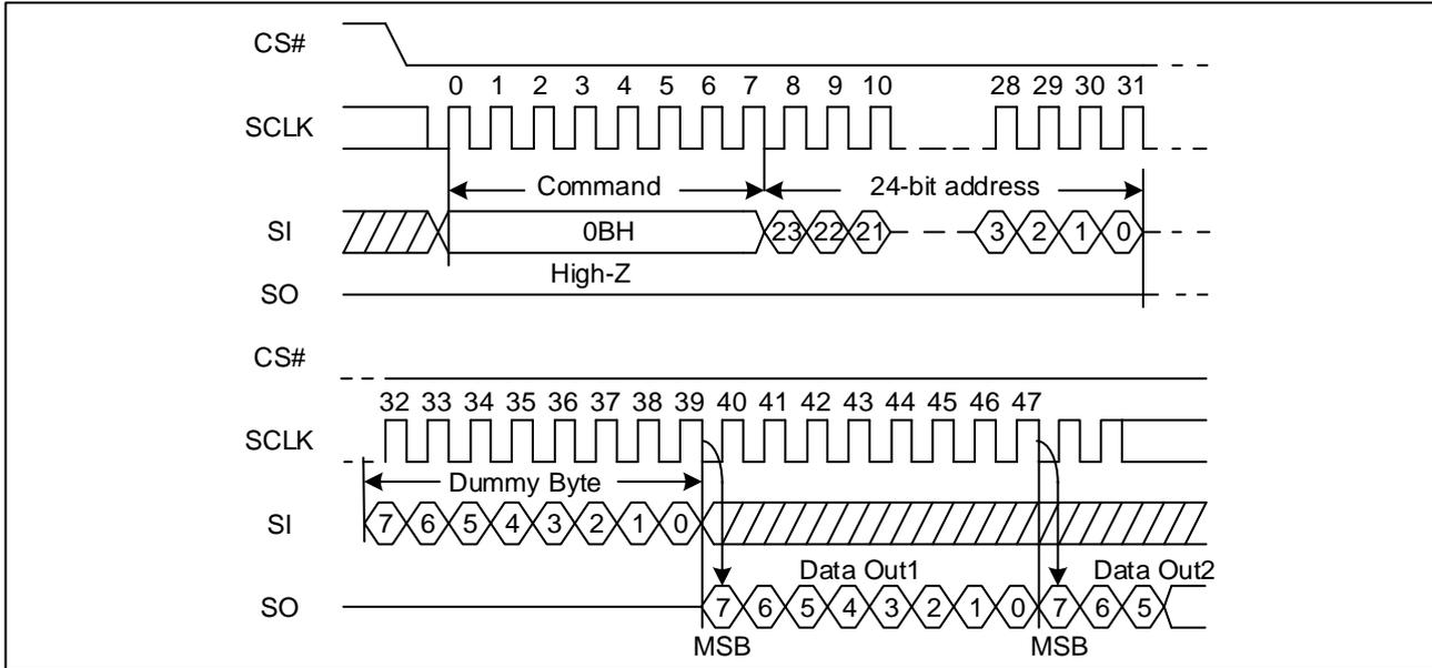
**Figure 15. Read Data Bytes at Higher Speed Sequence Diagram (QPI)**
