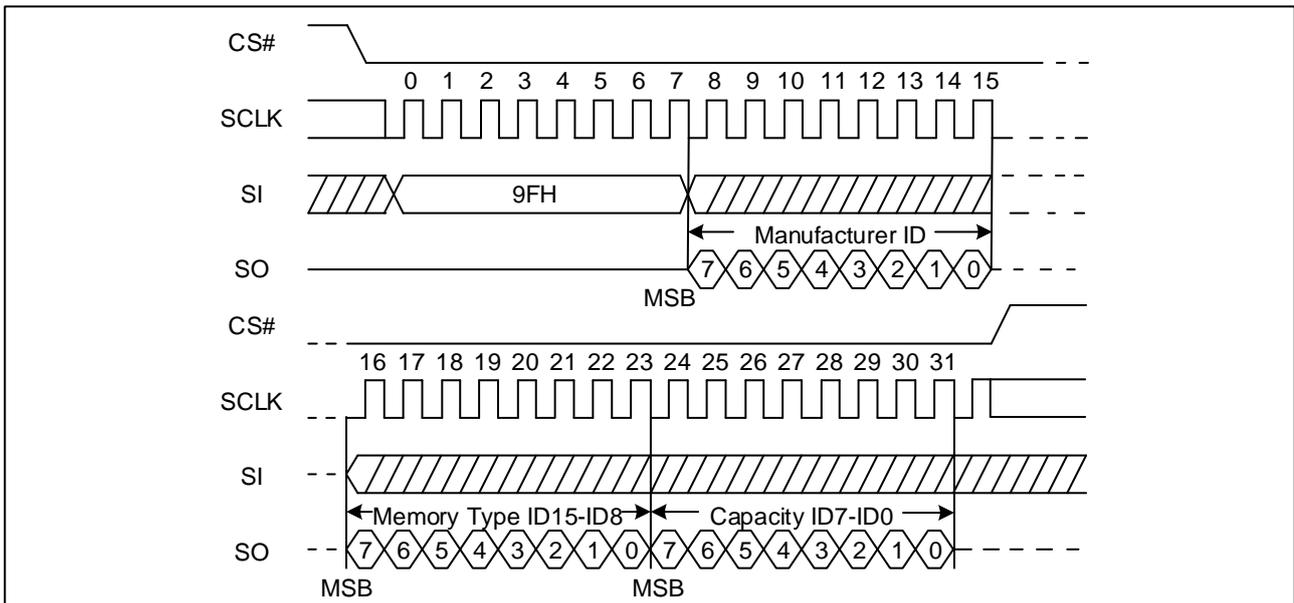
**Figure 43. Read Identification ID Sequence Diagram (QPI)**
