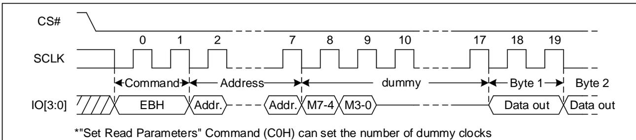
**Figure 22 Quad I/O Fast Read Sequence Diagram (M5-4 = (1, 0))**
