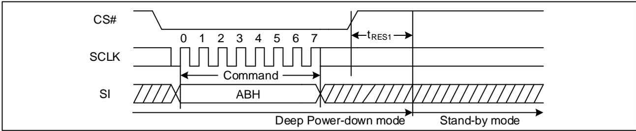
**Figure 57. Release Power-Down Sequence Diagram (QPI)**
