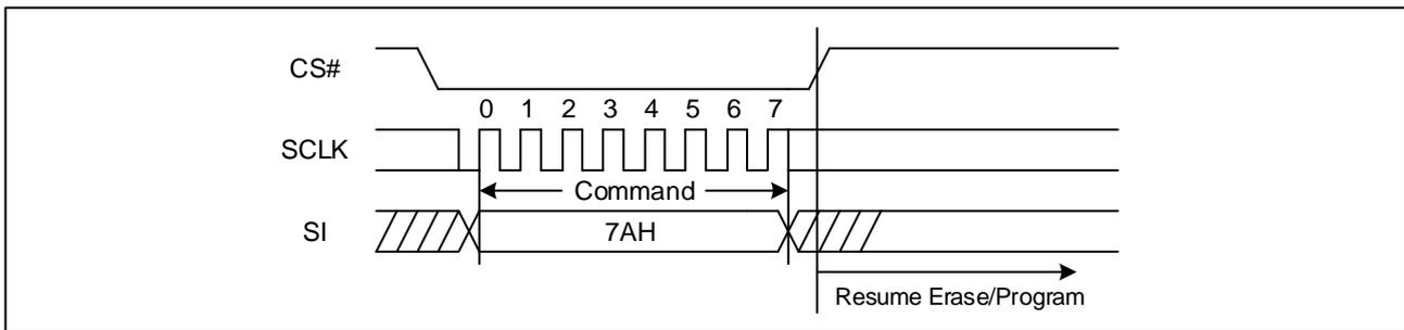
**Figure 53. Program/Erase Resume Sequence Diagram (QPI)**
