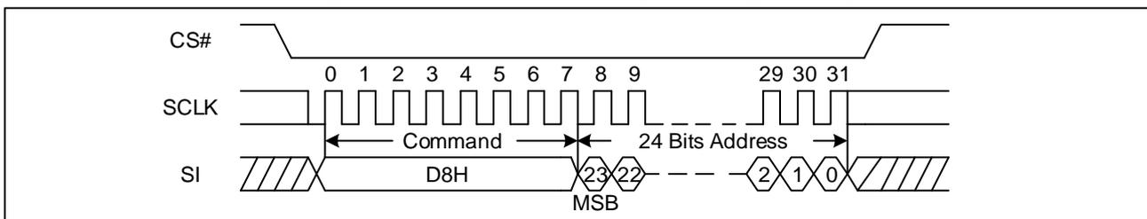
**Figure 37. 64KB Block Erase Sequence Diagram (QPI)**
