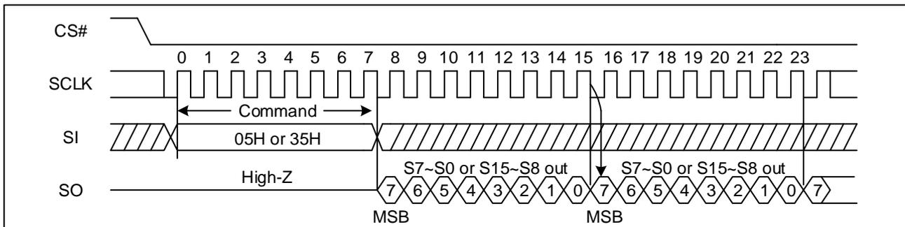
**Figure 8. Read Status Register Sequence Diagram (QPI)**
