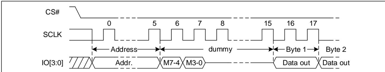
**Quad I/O Fast Read with “8/16/32/64-Byte Wrap Around” in Standard SPI mode**
