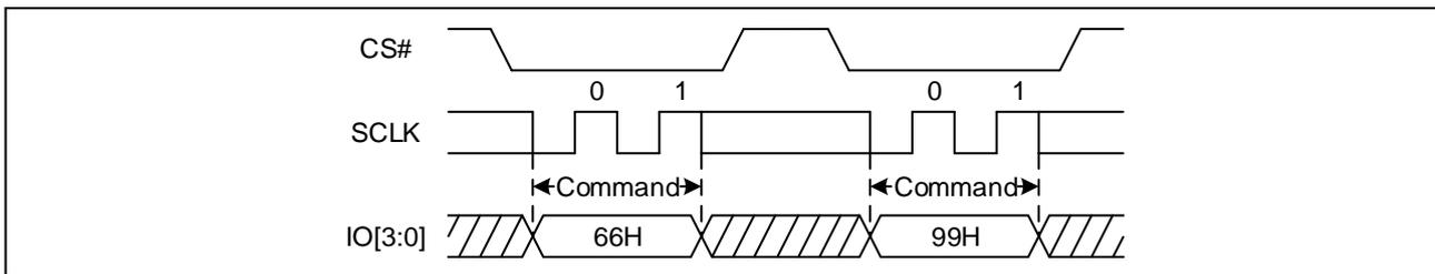
Note: Enable Reset (66H) and Reset (99H) commands cannot reset the device when the device is in Quad I/O DTR Continuous Read Mode. The only way to quit the Quad I/O DTR Continuous Read Mode is to set the “Continuous Read Mode” bits (M5-4) not equal to (1,0).
