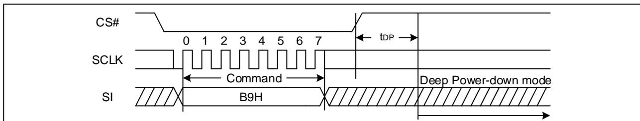
**Figure 55. Deep Power-Down Sequence Diagram (QPI)**
