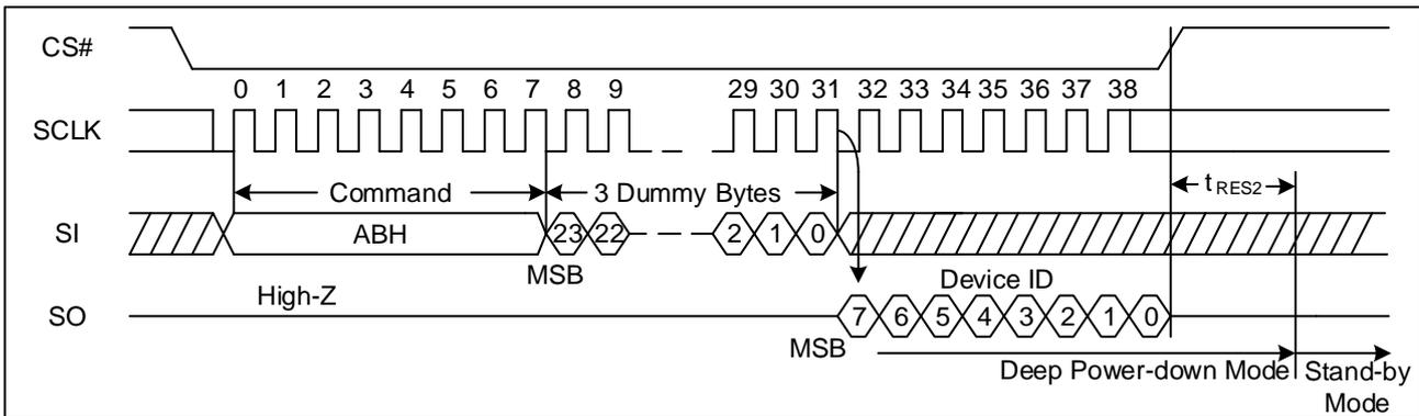
**Figure 59. Release Power-Down/Read Device ID Sequence Diagram (QPI)**
