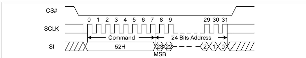
**Figure 35. 32KB Block Erase Sequence Diagram (QPI)**
