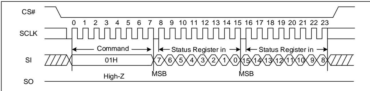
**Figure 10. Write Status Register Sequence Diagram (QPI)**
