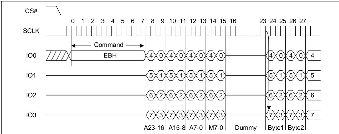
**Figure 21. Quad I/O Fast Read Sequence Diagram (QPI, M5-4 ≠ (1, 0))**
