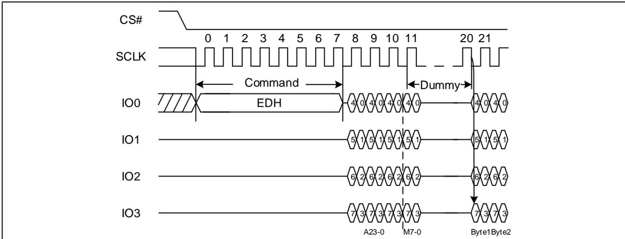
Figure 25. DTR Quad I/O Fast Read Sequence Diagram (QPI, (M5-4) ≠ (1, 0))
