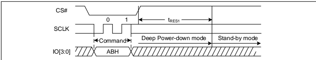
**Figure 58. Release Power-Down/Read Device ID Sequence Diagram (SPI)**
