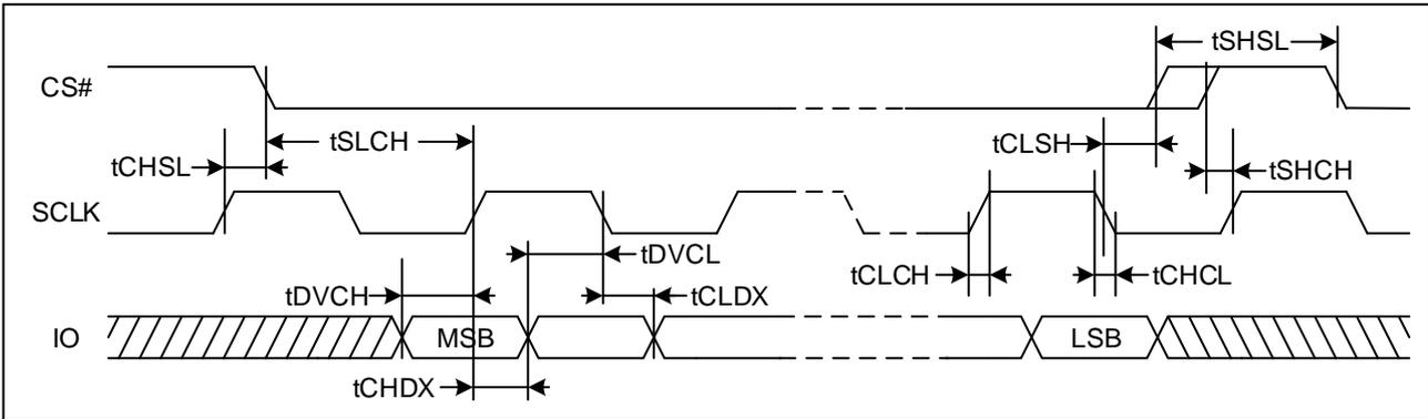
Figure 70. Serial Output Timing (DTR)
