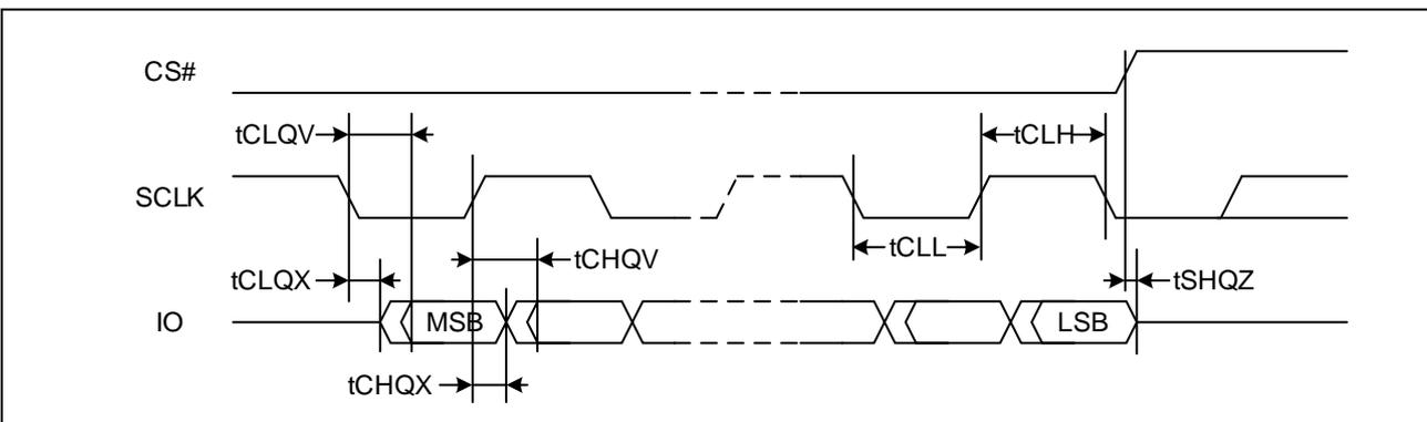
Figure 71. Resume to Suspend Timing Diagram
