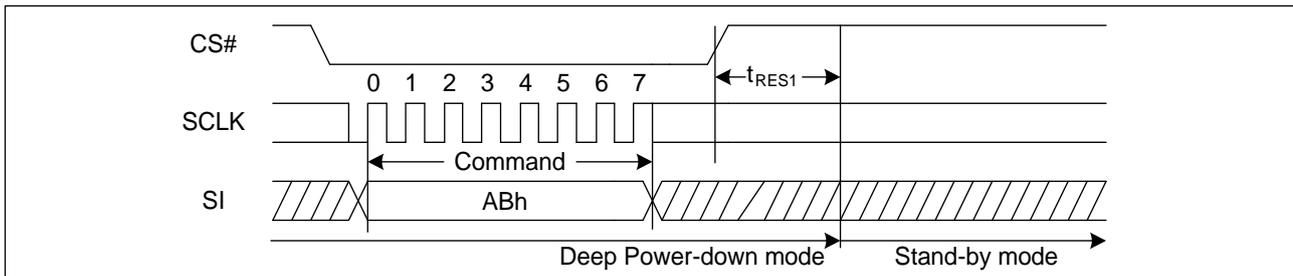
**Figure 36. Release Power-Down/Read Device ID Sequence Diagram**
