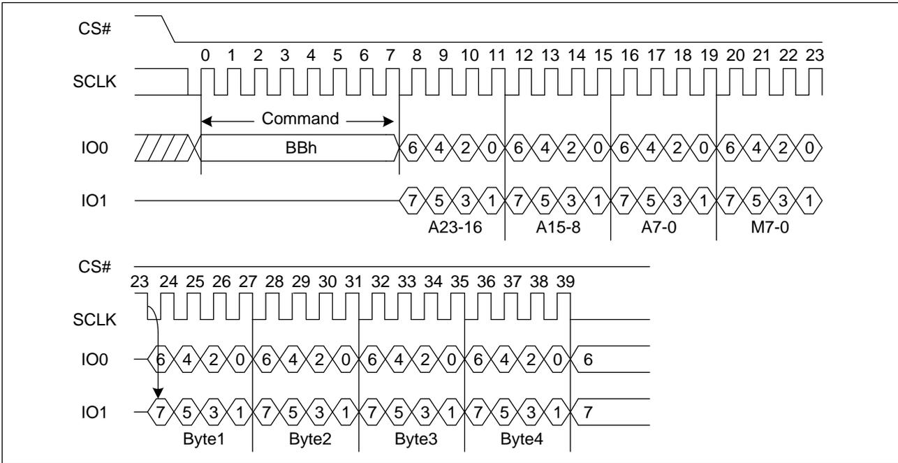
Figure 15. Dual I/O Fast Read Sequence Diagram ((M5-4) = (1, 0))
