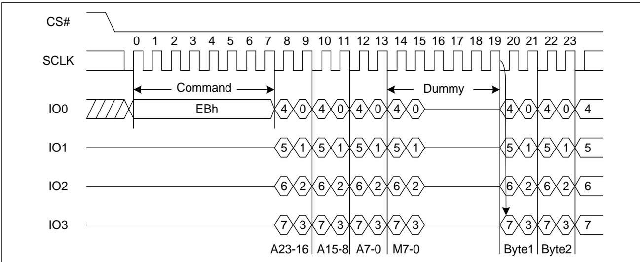
**Figure 17. Quad I/O Fast Read Sequence Diagram ((M5-4) = (1, 0))**
