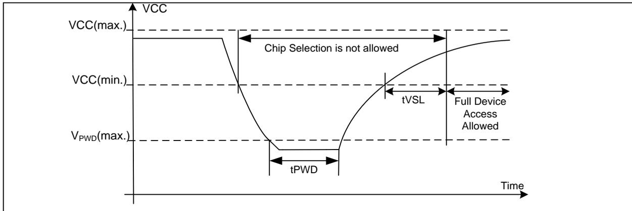
Table 11. Power-Up/Down Timing and Write Inhibit Threshold
